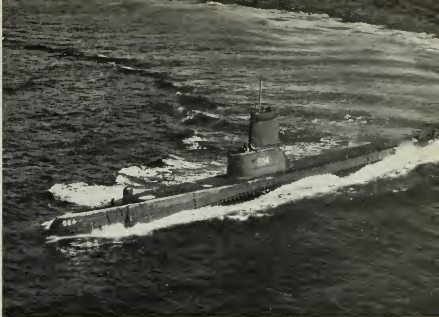
AFTER WW II Fleet-type subs were given new streamlined guppy look. Here, USS Pickerel (SS 524) makes way at sea.
